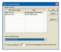
3. Select the printer that is connected to the selected Print Server. Click "OK". Note that in some cases, new printing jobs cannot be printed because the printer is already disconnected. It will cause unformatted messages to be printed out. "Keep connecting for 30 second(s) after printing has been finished (5-60)" is enabled by default. It will help to avoid this kind of situation.
